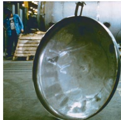
FIGURE 26: A warm formed vessel head of AL-6XN® plate. (Courtesy Gaston County Fabricators)
