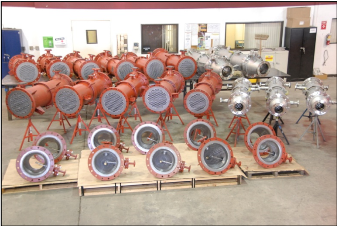
TANTALUM, HASTELLOY C AND 316L STAINLESS STEEL PHARMACEUTICAL CONDENSER WITH CIP SPRAY BALLS
