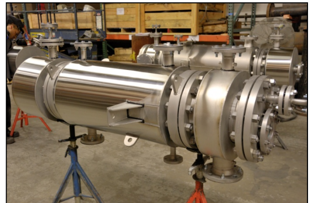
TANTALUM CONDENSER WITH INTEGRAL INSULATION, SIGHT GLASS, AND CIP SPRAY BALLS
