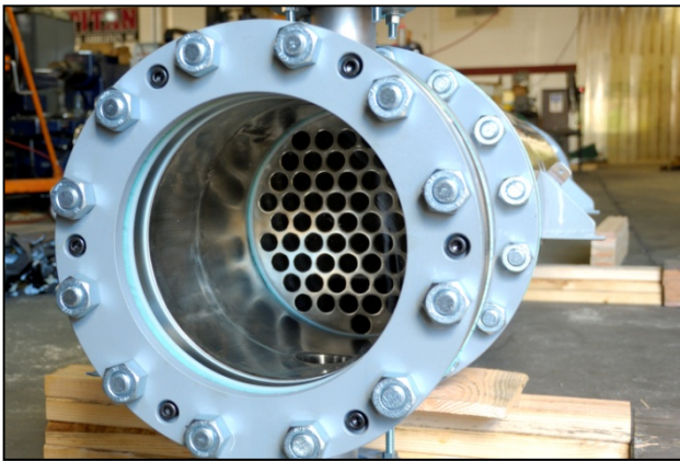
ALLOY C CONDENSER WITH TUBESIDE POLISHED TO 20 RA AND SIGHT GLASSES ON BONNET FOR VIEWING CONDENSATION
