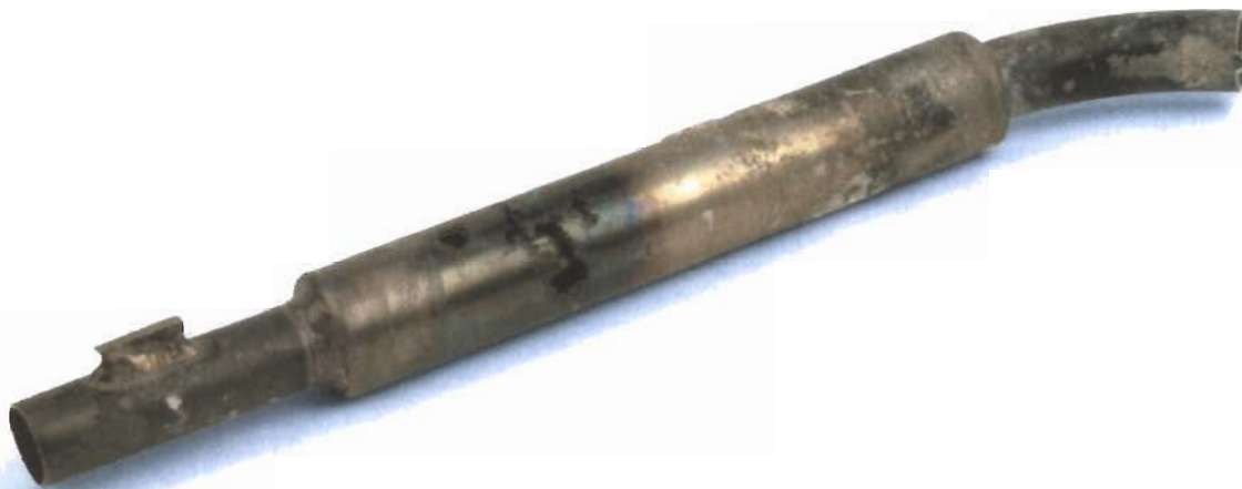
Fig. 7: "Sacrificial" solution level protector exhibiting pitting corrosion
